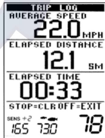
STOP Resets timer ON-OFF Enables timer
